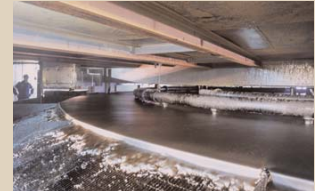
Suncor's oil sands primary extraction plants separate raw bitumen from the sand in giant separation cells.
